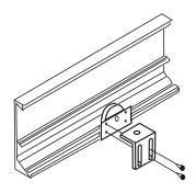
According to the length of faceplate, fix the two fixing lugs on the side of
